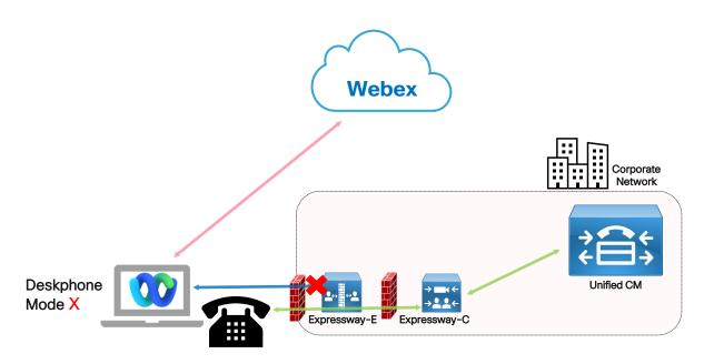
When running outside the corporate network, Webex App cannot control a Cisco Deskphone via CTI. Mobile Remote Access does not support CTI connections
