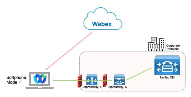
When running outside the corporate network, Webex App can register to Unified CM in softphone mode (SIP) via Mobile Remote Access
