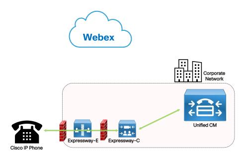
When running outside the corporate network, a Cisco IP Phone can register to Unified CM (SIP) via Mobile Remote Access
